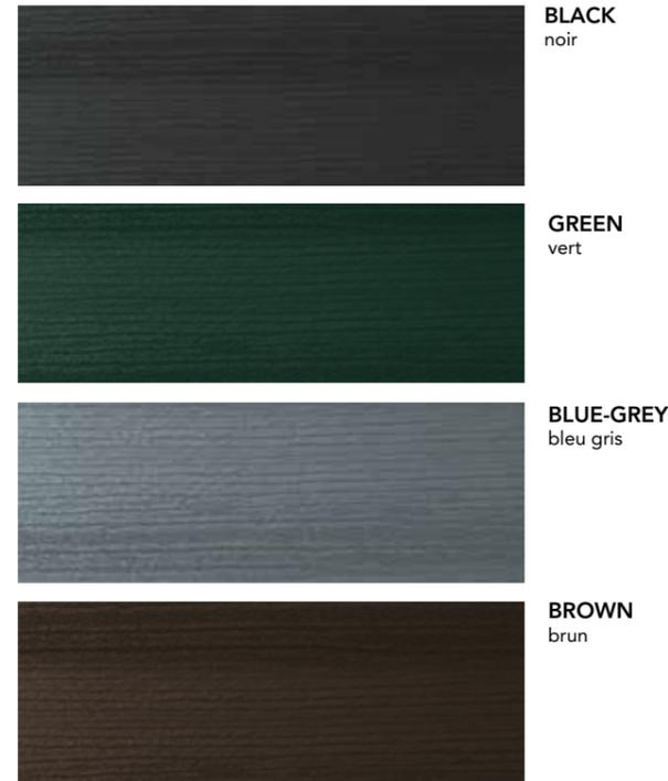
The name ARDESIA identifies a polyester-painted steel with a wrinkled surface. It is specifically designed for roofs with a "false tile" appearance or in any case with 0 gloss properties; the prepainted product can be compared to the **Marcegaglia MP4 system**, with a predicted average life of at least **10 years**.
